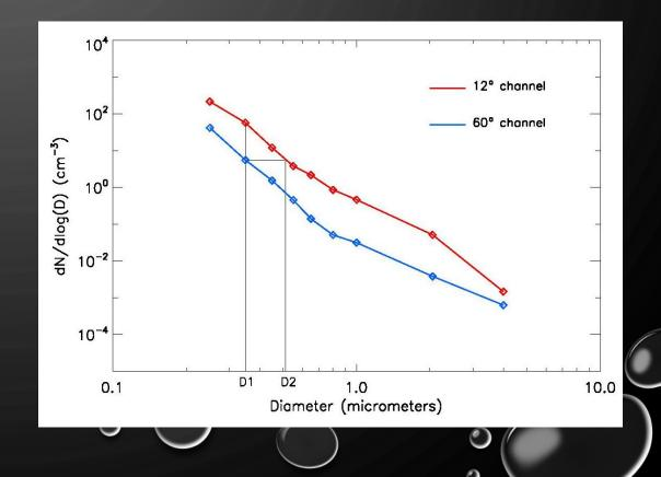
The 12°/60° ratio ("speciation index") is compared to charts obtained in laboratory for different families of particles:
