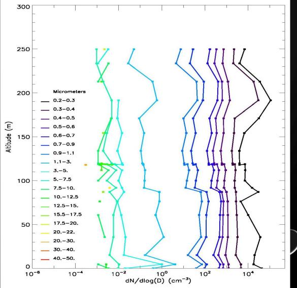
O Counting measurements can be converted to PM 2.5 and PM10 mass (μg/m<sup>3</sup>)
